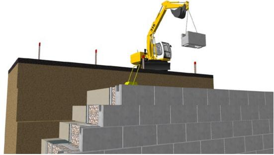
▶ Continue the installation of MaxumStone® big block gravity retaining wall as per the design provided. Cross section drawings will show you where the units are placed in order of depth.
