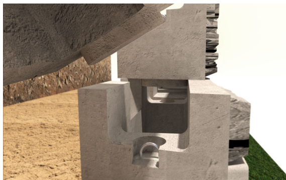
BLOCK INSTALLATION WITH SECURELUG
